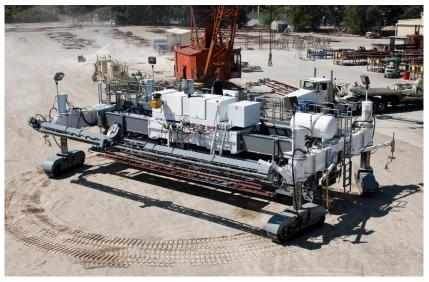
The S1500 is equipped with counter-rotation capability where the operator can quickly re-orientate the S1500 crawlers into the counter-rotate position and rotate the machine 360 degrees within the machine's overall width. Counter-Rotation is just one of the pre-programmed steering modes available with the S1500 controls, along with crab and coordinated steer, front and rear only steer.
