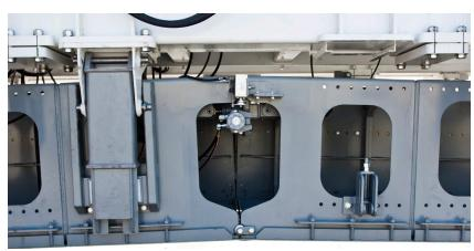
The optional Paving Kit Crowning Section is provided with a hydraulic motor driven, dual screw jack system that holds the crown position without drift. A digital readout of the crown angle is provided at the operator console. Computerized Crown / Transition Control system is also available as an option.
