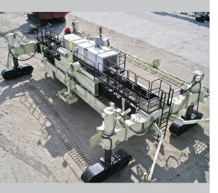
Deep section, fabricated, tube type construction of the double telescopic tractor frame design allows paving widths from 18 ft. (5.5 m) to 42 ft. (12.8 m). The machine telescopes 12 ft. (3.6 m) on either side of the 18 ft. center module for a total telescopic ability of 24 ft. (7.3 m) With the addition of optional bolt-in frame sections, the total possible paving width is 52.5 ft. (16 m).
