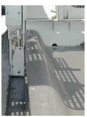
The terminal pan sections on the Paving Kit are provided with edge overbuild adjustment to help compensate for edge slump. The terminal pans can be substituted with other optional integral curb and gutter mold cross sections.
