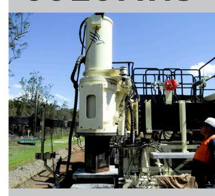
G&Z's precision built, square-to-round style jacking column design with built-in replaceable bronze wearing parts that prevent sticking allow for the most positive steering control in the industry. This design also offers years of precise, maintenance free use.
