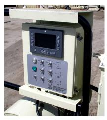
visibility of the paver's concrete spreading operation. The control desk includes a lock out / power switch locate inside the control desk, an aluminum cover for weather and vandal protection and an emergency stop.
