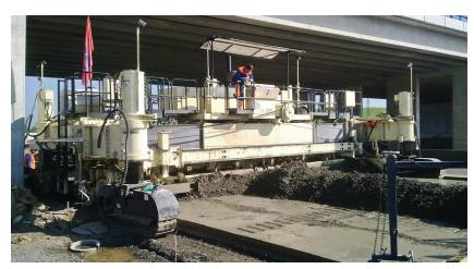
transport to reduce the load weight due to trailer weight limitations. With a special trailer capable of hauling long, heavy loads, the paving kit may be left attached. The S1500 can easily walk and steer onto a standard 8 ft. (2.5 m) wide trailer with a transport width of under 12 ft. (3.5 m). There is no switching of hoses required on the crawler tracks and the crawlers are automatically kept parallel for steering.
