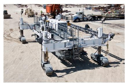
90 Degree Steering Mode allows the four crawler tracks to be turned perpendicular to the paving direction with a flip of a switch. The operator is provided with limited steering range in this mode. 90 Degree Steering reduces the size of hand pours, dramatically increases on site paver maneuverability and helps speed width change and self-loading for transport.
